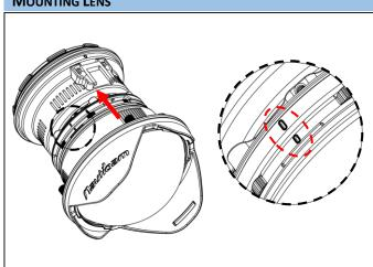
Align the "I" mark on the lens with the "I" mark on the Converter and then push it in.
