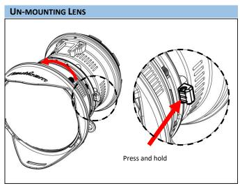
Press and hold the RED lens release button and then turn the lens anti-clockwise.
