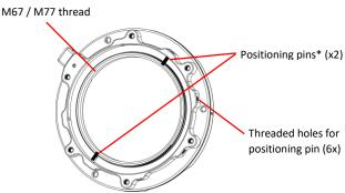
\*There are two alignment pins at the bottom of the holder, by relocating the two screws to the threaded holes around the holder, the position of the holder can be changed.
