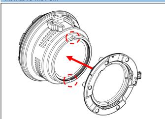
Align the two positioning pins on the back of the converter with the slots on the front of the port. Fasten the converter on the front of the port with the tool provided.
